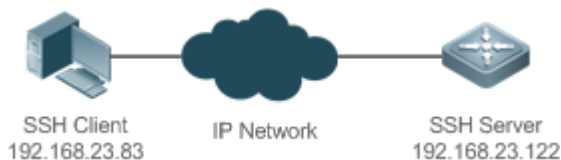
Figure 1-4 Network Topology for Public Key Authentication of SSH Users
